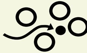
For contaminants 0.2 to 2  $\mu\text{m}$  in size, interception is the predominant coalescing mechanism. These contaminants conform to the stream line of the air flow and are the most difficult to remove because they can pass around filter fibers and escape from the filter uncollected. In general, efficiency of the "intercept" mechanism
