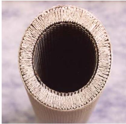
Right: This outer layer of the 7CVP consists of a dense matrix of glass fibers. The coalescing outer layer provides highly efficient aerosol removal with very low pressure drop.
