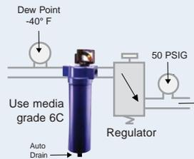
Any compressor with aftercooler, two-stage and double coalescing and a regenerative-type desiccant dryer. Air intended for use in applications involving rapid expansion of compressed air, critical instrumentation, high purity gases, computer chip drying, etc. CAUTION: This air is too dry for respiratory use.
