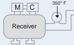
Any small compressor with no aftercooler, air intended for intermittent, general use.
