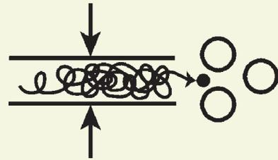
forces. Liquid droplets, however, migrate gravitationally down the filter fibers, joining other droplets to form larger masses of liquid which can be drained from the system. While the rate of diffusion activity increases with heightened temperature and pressure, contaminants of this size exhibit random motion – and are subject to diffusion coalescing – even under non-turbulent, low velocity flow conditions.
