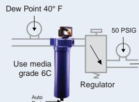
Any compressor with aftercooler, 2-stage coalescing & refrigerated dryer. Air intended for use with air-gauging, air conveyors, spray-painting, food processing, instrumentation, blow molding, cosmetics, film processing, bottling, pharmaceuticals, dairy, breweries, medical, robotics & close tolerance valves.
