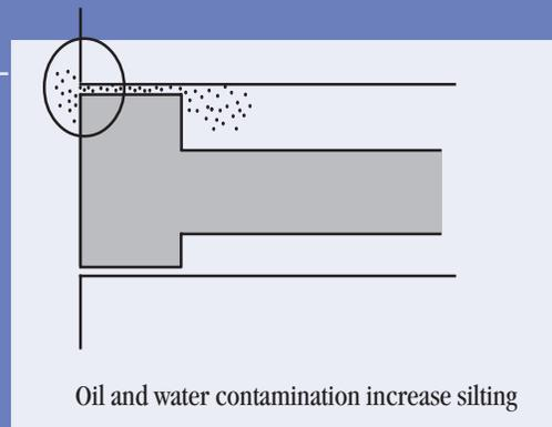
Oil and water contamination increase silting
