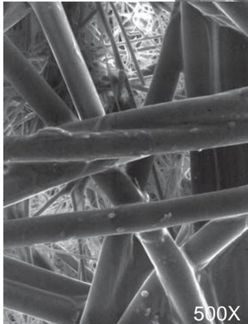
Left: This inner layer of the 7CVP effectively traps dirt particles, protecting and extending the life of the outer layer.
