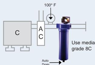
Any compressor with aftercooler & 2-stage coalescing. Air intended for use with lubricated control valves, cylinders and parts blow-down, etc.
