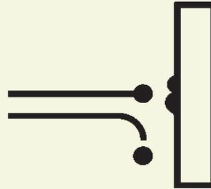
Contaminants 2  $\mu\text{m}$  and larger are removed by the direct impact method because they have sufficient mass and develop enough momentum to leave the air flow stream line. These contaminants collide with the filter media, a coalescing process termed inertial or direct impactation.
