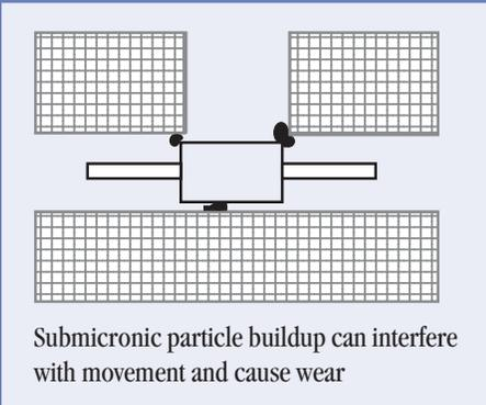
Submicronic particle buildup can interfere with movement and cause wear
