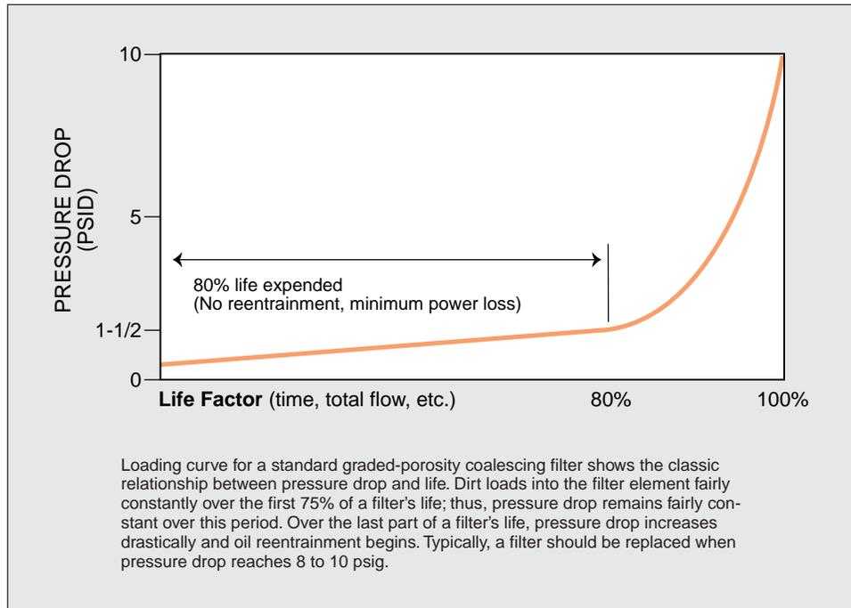
*Increasing pressure drop is a sign that the filter is becoming clogged and its efficiency could become impaired*
