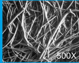
Grade 2 filters are used for extremely fine particulate and “last trace” aerosol coalescing filtration; for lighter molecular weight gases and aerosols at higher pressures.
