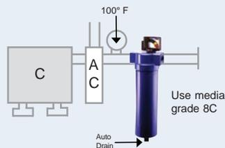
Any compressor with aftercooler. Air intended for use with lubricated air tools, air motors, cylinders, shot blasting, non-frictional valves.
