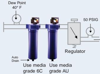
Any compressor with aftercooler, 2-stage coalescing, refrigerated dryer & carbon absorber. Air intended for use as industrial breathing air & decompression chambers. CAUTION: Always use high temperature synthetic lubricants & monitor (alarm for carbon monoxide concentrations exceeding 20ppm). This system will not eliminate toxic gases!
