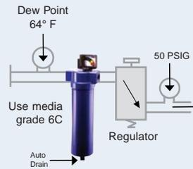
Any compressor with aftercooler, 2-stage coalescing & deliquescent dryer. Air intended for use with general pneumatic systems, body shop spray painting and components sensitive to high moisture content.
