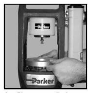
4. Place proper die ring on top of the selected die. See Parker PFD Catalog 4660 for proper die ring selection.
