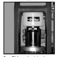
5. Slide pusher into place onto shoulder bolt.
