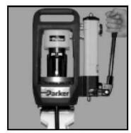
While holding hose and fitting into position on die step, begin pumping hand pump until die ring contacts base plate.
